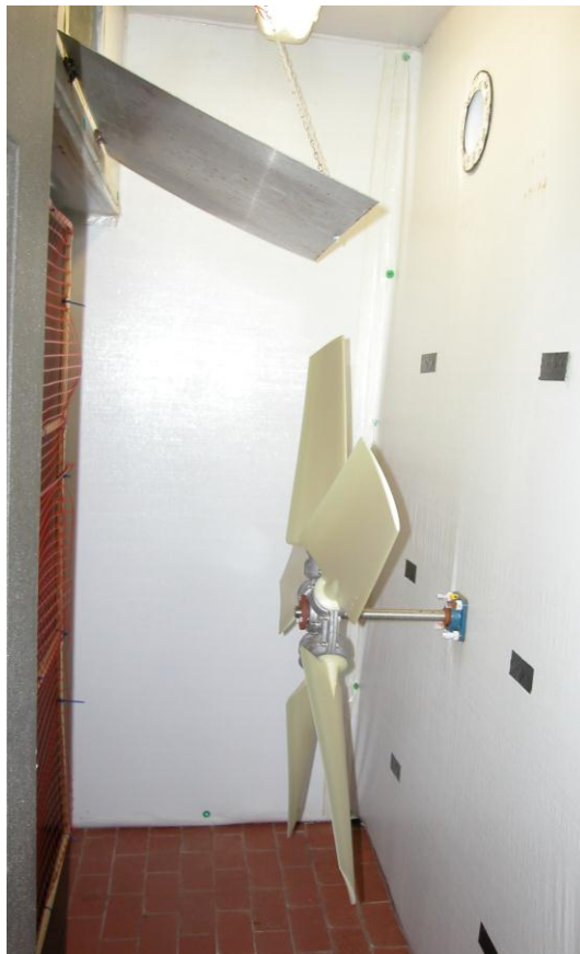
Figure 53. Optimum baffle angle at -15 degrees from the horizontal.
