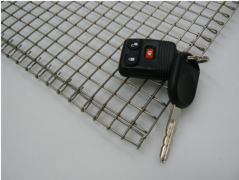
Figure 49. Detail of dehydrator shelf or tray showing “hemmed” edge, which added rigidity to the shelf and concealed the cut edge of the wire cloth.
