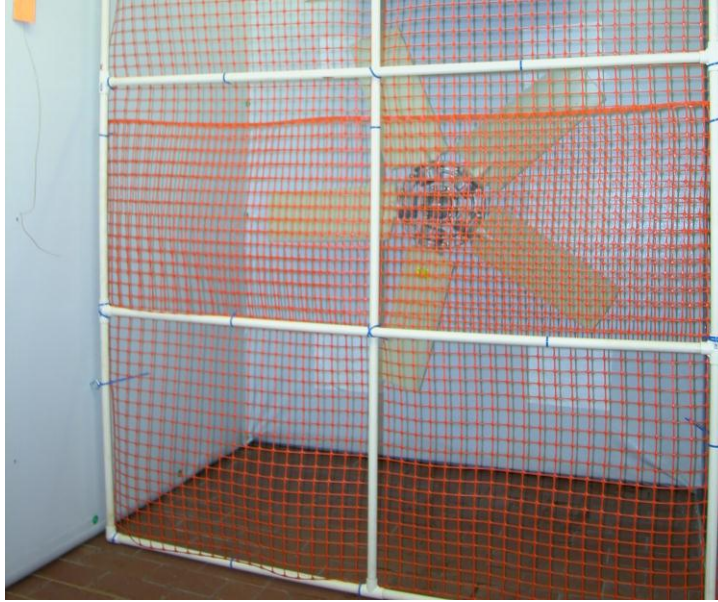
Figure 54. Guard protecting product from fan blades. Guard is constructed of PVC tubing reinforced with conduit.
